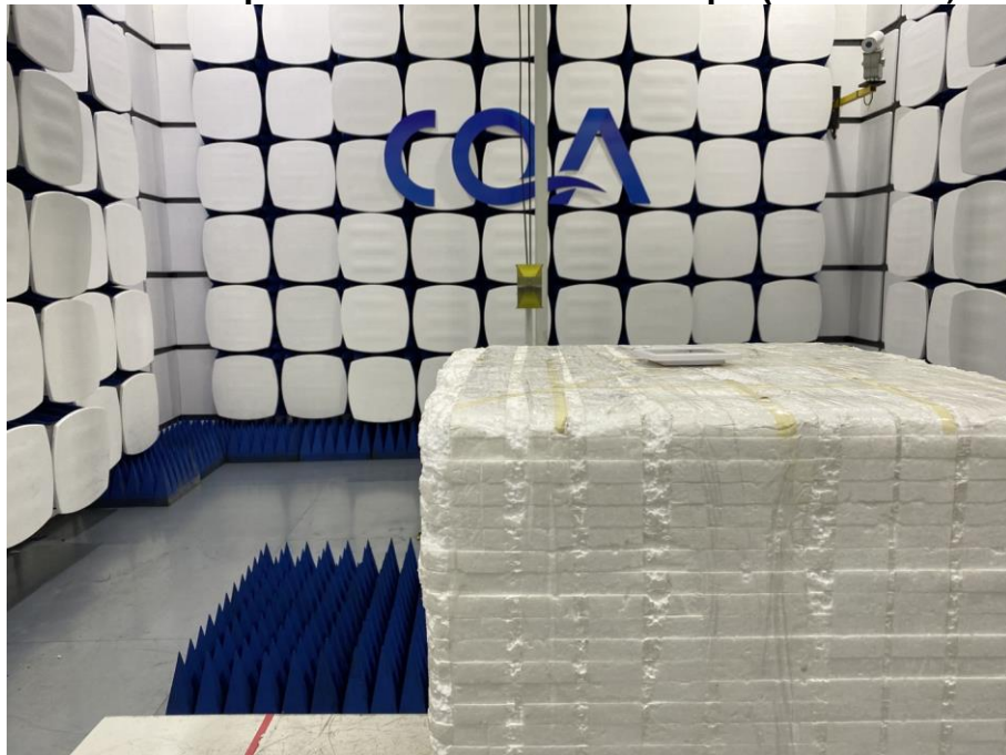
Radiated spurious emission Test Setup-2(Above 1GHz)
